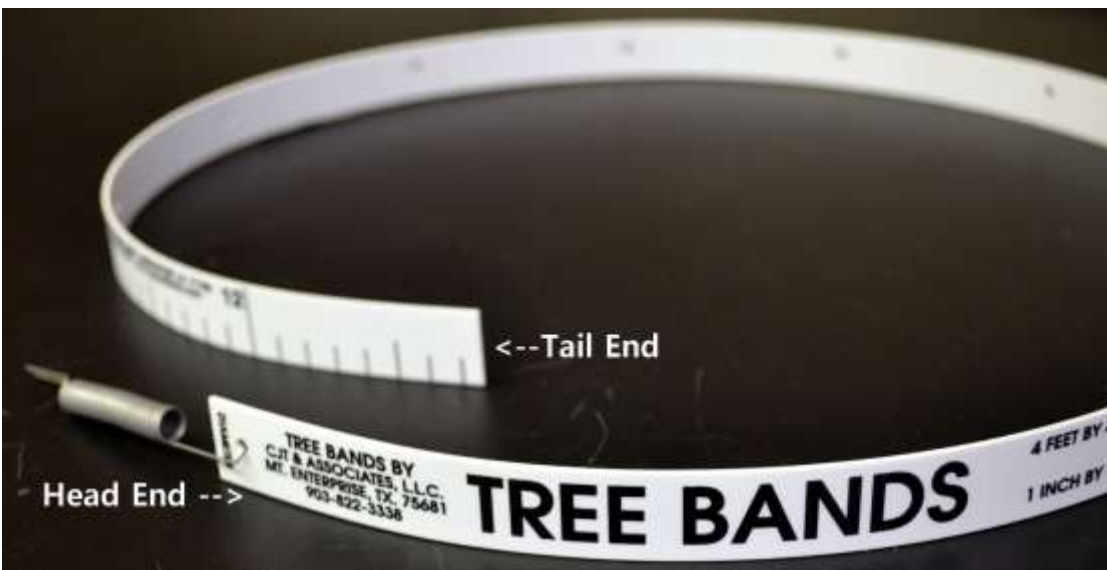
Fig 3. Parts of the dendrometer: Head End, Tail End, and Spring.
