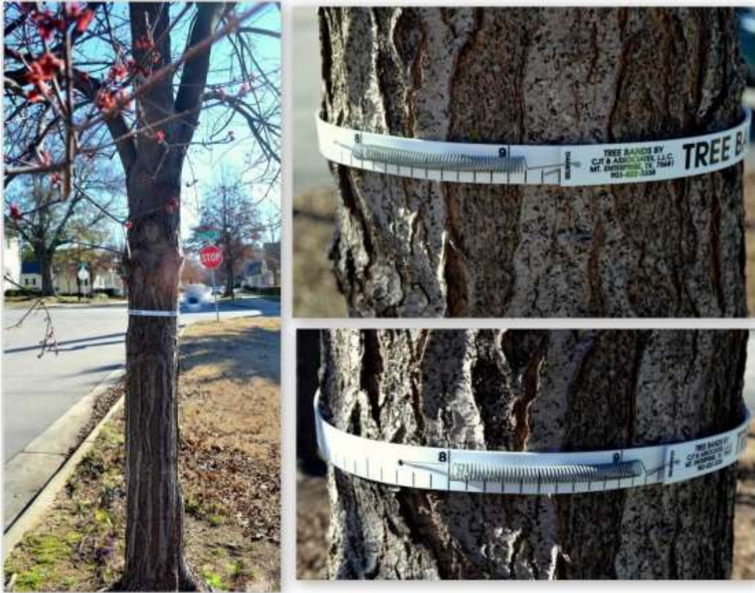
Fig. 2 Correct placement of the dendrometer. This red maple has a DBH of 9.3 inches, as indicated by the dendrometer. When uploading your data, include a photograph like those on the right that show your tree's DBH.
