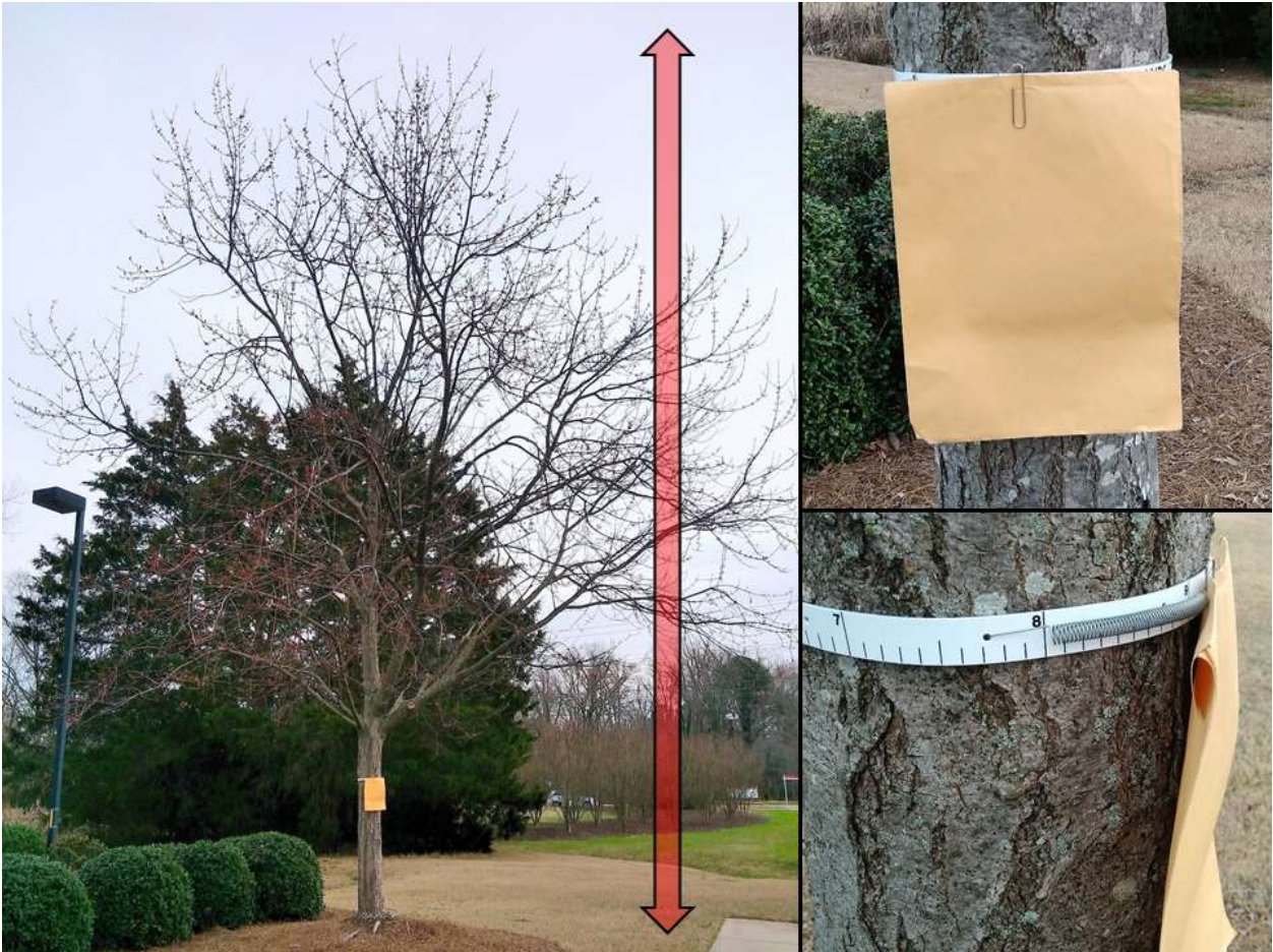
Fig. 4. Placement of envelope, and example photograph of tree with envelope. Be sure to capture the entire height of the tree in your photograph. In this example, we used a paperclip to hold the envelope to the dendrometer. When hanging the envelope, take care not to disturb the dendrometer. If you don't have the envelope use a ruler or yard stick.
